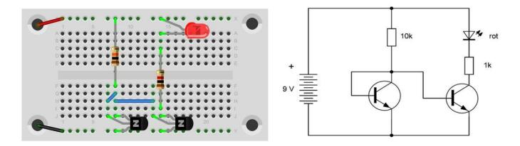
In this circuit, the base and collector of the left transistor are directly connected to the base of the right transistor. That means the same base voltage, and with exactly the same transistors, the same collector current. The collector current of the left transistor is determined by its collector resistance of  $10~\text{k}\Omega$ . The same current then appears "mirrored" at the right transistor. This circuit is therefore also called a current mirror.
