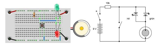
Let's get on, we can do even better! Turn off the battery and keep the button open. If you then lightly tap the membrane of the piezo speaker, flashes of light are created. The piezo transducer now works as a microphone or a generator.
