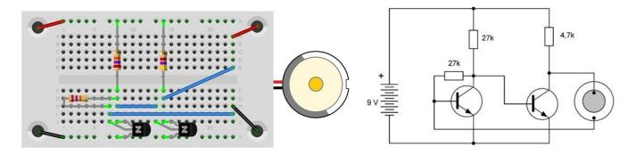
The circuit with two bipolar transistors forms an astable flip-flop. The piezo speaker is also the frequency-determining capacitor. In addition, the frequency is influenced by the loudspeaker's own resonance, which can be changed by reflections on a hard surface or by touching it.
