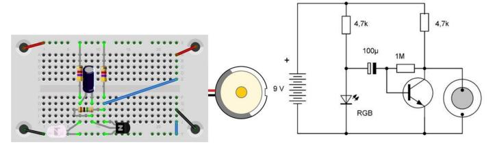
In addition, this circuit has a transistor amplifier and a piezo speaker. You can always hear tones from the speaker when there is a transition from one color to another, resulting in mixed colors.
