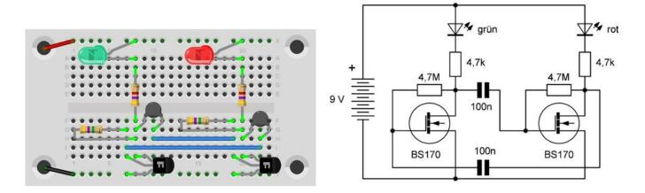
This circuit is called an astable flip-flop. It also knows two stable states, but only for the relatively short time in which the capacitors recharge to the new state. The 4.7 M $\Omega$  resistors were chosen to be large enough so that the relatively small 100 nF capacitors are charged sufficiently slowly.
