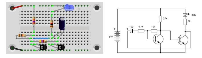
A particularly small series resistor of 1 k $\Omega$  was used in this circuit in order to achieve high brightness. At the same time, however, this also means greater consumption. You can therefore also test resistances up to 10 k $\Omega$  so that the battery lasts longer. And the capacitor can also be changed. With an electrolytic capacitor of 100  $\mu$ F, the flashing becomes ten times slower.
