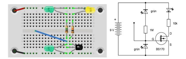
In this experiment, two LEDs are connected to the gate as reverse-biased photodiodes. If you only light the upper one, the transistor will conduct and turn on the yellow LED. If only the bottom one is lit, the yellow LED goes out. So the circuit works like a switch that is controlled by light and shadow.
