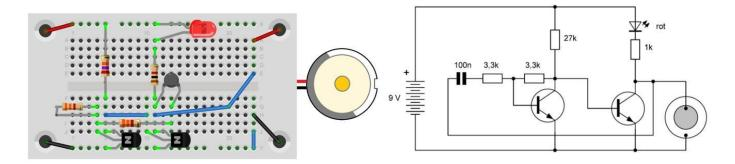
The LED appears to glow evenly and constant, but it actually turns on and off about 300 times in a second. If you let your eyes wander quickly over the experiment or move the entire structure, you can see that the glow dissolves into individual lines.
