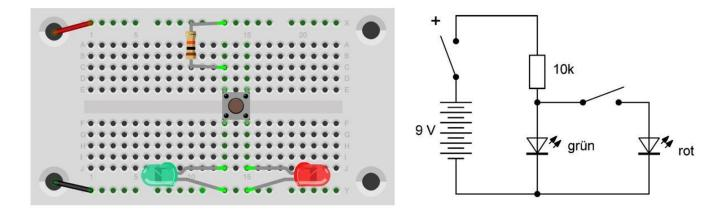
The explanation can be found in the different specification of the two LEDs. As with any diode, the current only increases steeply with increasing voltage above a certain voltage. This voltage is higher for the green LED than it is for the red one. So, when the current limited by the resistor flows through the red LED, the voltage drops so much that this voltage is no longer sufficient for the green LED. A test with two green LEDs shows it: Both will light up in parallel.
