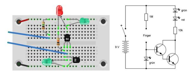
The circuit has another function as well. If you touch the two free cables with your finger, the LEDs also switches on. A very small, imperceptible current then flows through the fingers, which the transistors amplify to such an extent that the LEDs are switched on. For use as a touch switch, the left green LED is not required and could be removed.
