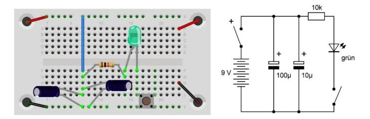
The electrolytic capacitors are used here for energy storage. If you close the switch on the battery compartment, they will be charged. Then you disconnect the battery and press the button switch. The LED lights up for up to 10 seconds and slowly fades away. You can see how the stored energy is consumed.
