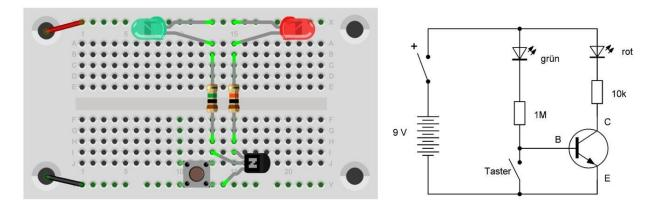
If you now press the button, the green LED stays on, but the red LED goes out. The control current is going to ground when the switch is closed, i.e. the base current is switched off, so that no more collector current flows. But as soon as you release the button, the red LED switches on again.
