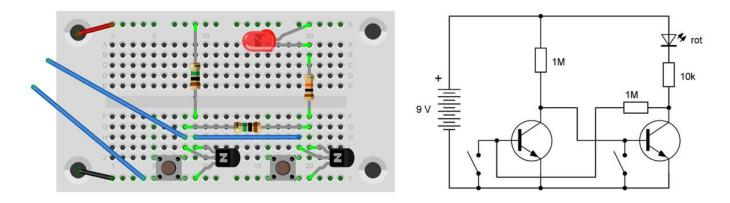
If you look closely, you will see a weak residual light in the off state. Then still the low base current of the left transistor flows through the LED. In the comparable circuit with field effect transistors, on the other hand, the LED was completely off. Here you can see the crucial difference again: Bipolar transistors are controlled by a current, while unipolar transistors are controlled by a voltage.
