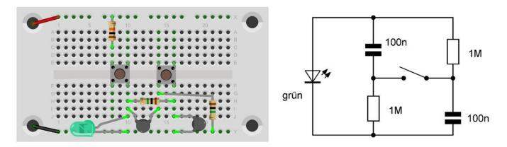
For a first test there is the left button and an additional resistor. Both of them are not part of the actual experiment and are therefore not included in the circuit diagram. But you can briefly press the left button to quickly charge the capacitors. Then you press the right button and you get the flash of light you're looking for. This makes it clear as a test, that everything was set up correctly.
