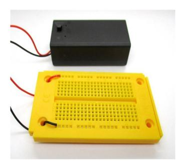
The battery compartment has tinned wires at the end, that could easily wear out if you keep plugging them into the board. In order for these cables to remain stable for all experiments, they should be fed through the mounting holes. To do this, you have to pierce the foil with a needle.
