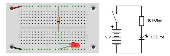
The patch panel has 230 contacts in the central area, each of which is conductively connected by vertical strips with 5 contacts. In addition, there are 40 contacts for the power supply on the edge, which consist of two horizontal contact spring strips with 20 contacts each. The patch panel thus has two independent supply rails, which are used here for the positive pole (top) and the negative pole (bottom) of the battery.
