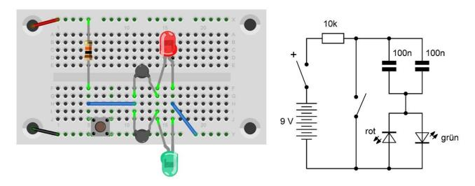
The experiment shows how these capacitors are charged and discharged in very short moments. It shouldn't be too bright in the room. When you press the button, the red LED flashes because the capacitors are being discharged. If you release the button, the capacitors are charged again, and the green LED lights up briefly. Taking out a capacitor gives weaker flashes. Two 100 nF capacitors in parallel behave like one 200 nF capacitor.
