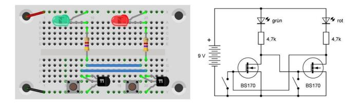
This circuit is also called a multivibrator or flip-flop because the state always flips to one side. In this case it is an RS flip-flop, which stands for the two states reset and set. This circuit shows how a data memory is structured in a computer. However, only one bit is stored here. Larger memories contain a lot of MOSFETs.
