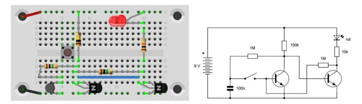
You can see the similarity to the RS flip-flop. But this time there is a capacitor that charges up to the voltage at the collector of the left transistor with a small delay. When the base voltage is high, the collector voltage is low and vice versa. Therefore, when the contact closes, a change of state is forced. Such a circuit is called a toggle flip-flop. It is also a frequency divider. If you press the button ten times, the LED only lights up five times.
