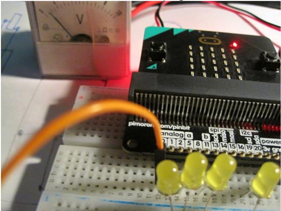
*Digital and analog (PWM) outputs from Mycobit*
